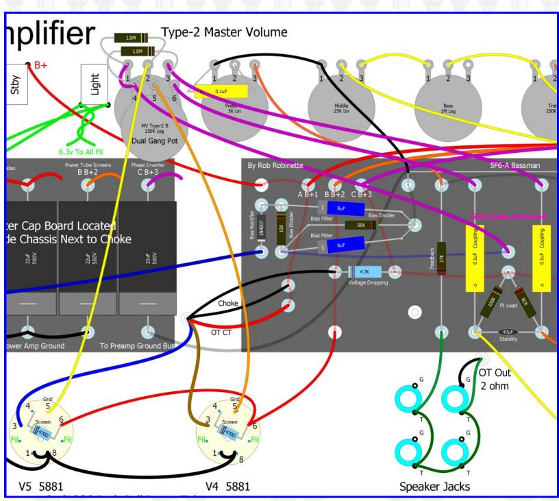
The 1.8M resistors on the Master Volume pot reduce the pot resistance to 220k and add a failsafe path for bias voltage.
