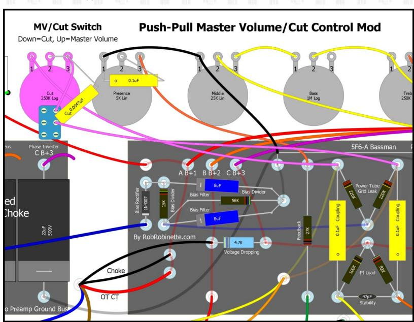
You can turn a Cut Control into a Trainwreck Type-3 Master Volume by simply jumpering around the Cut Cap. Use a 250KA push-pull pot and you can push the pot down for Cut Control or pull it up for Master Volume.
