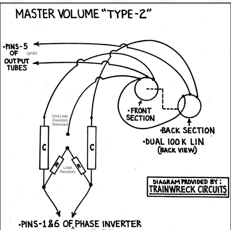
LTP TUBE (OR PINS 6 & 8 OF A CATHODYNE PHASE INVERTER)
