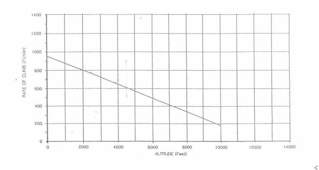
Note: In hot weather, reduce the rate of climb by 20 feet per minute for every 5°C above the standard temperature at the altitude in question.
