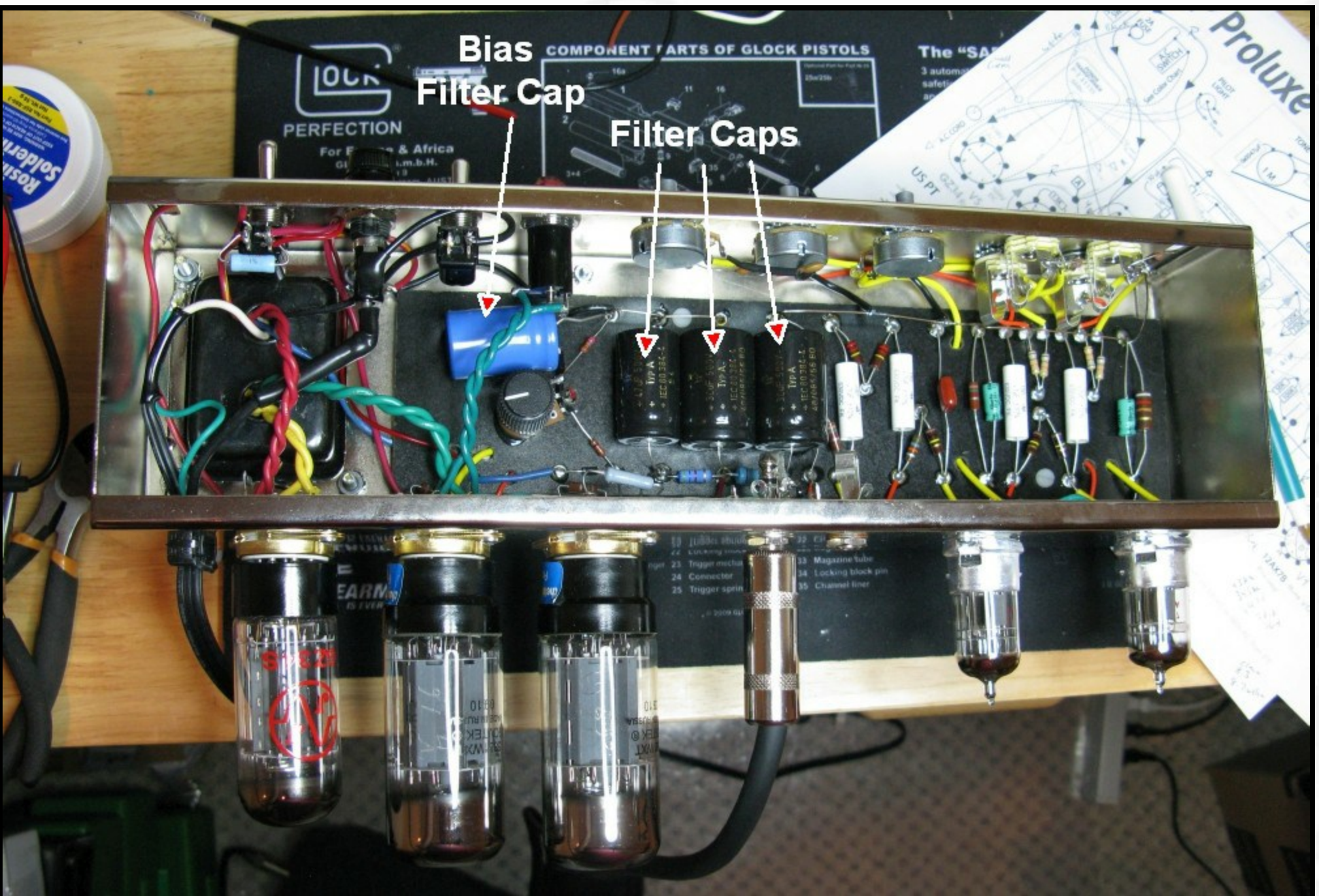
This is a 5E3 Deluxe with fixed bias so it has a bias filter cap (big blue cap above).
