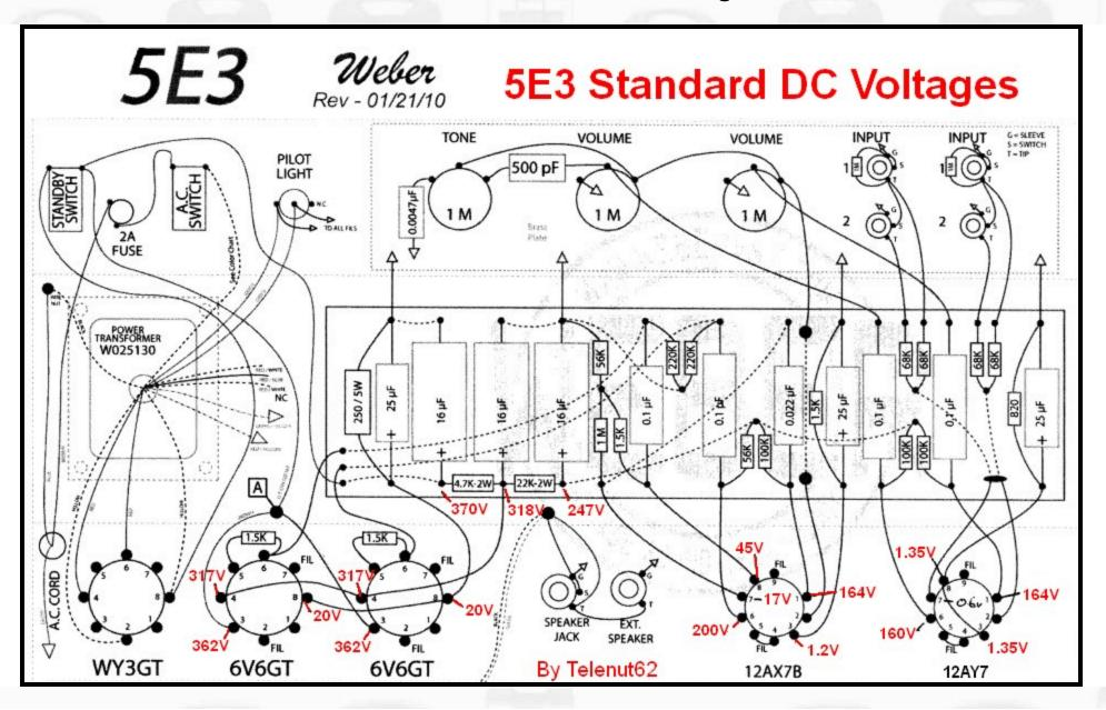
**Your voltages may be lower than these with the amp plugged into a light bulb limiter**. Note the V2B phase inverter (pins 6, 7 & 8) voltages are different than V1A, V1B and V2A gain stages. Diagram by Telenut62
