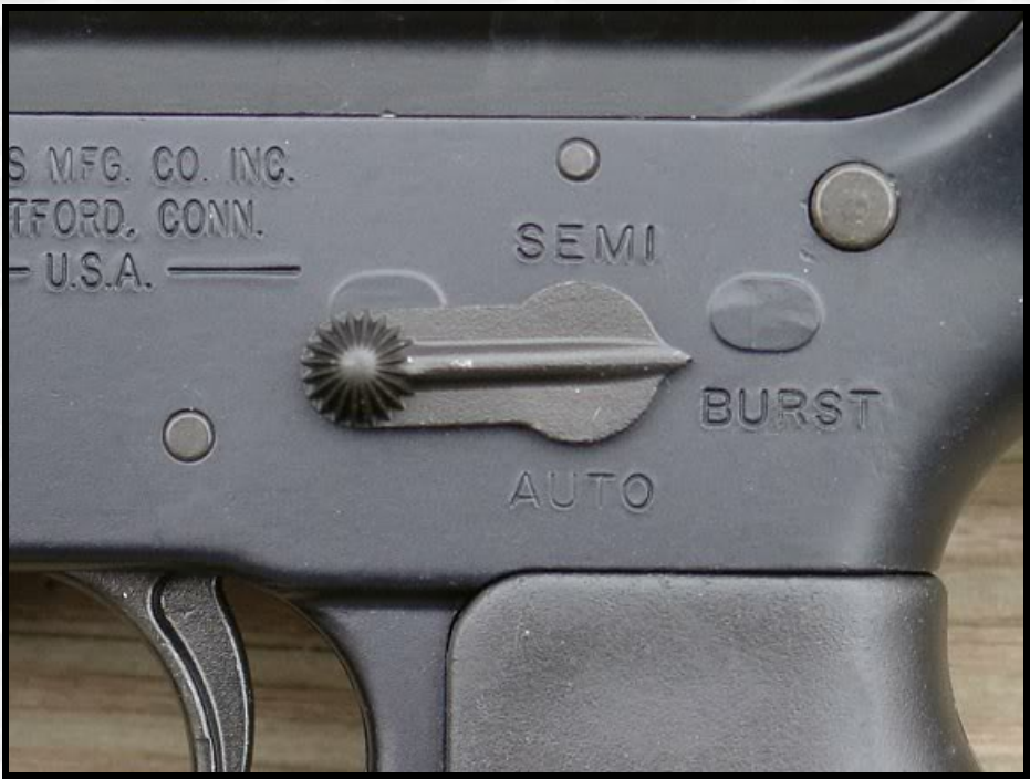
Note the filed-down selector stops.
