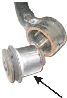
Factory bushing metal shell must be pressed out of upper control arm for Energy Suspension polyurethane bushings to fit properly.
