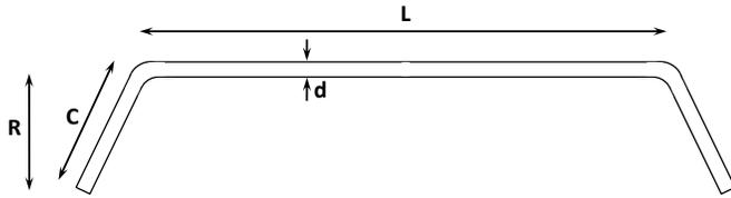
**Figure 3.** Parameters of a torsion bar with splayed arms
