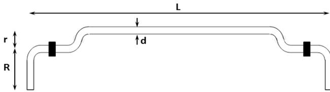
**Figure 4.** Parameters of a torsion bar with central offset
