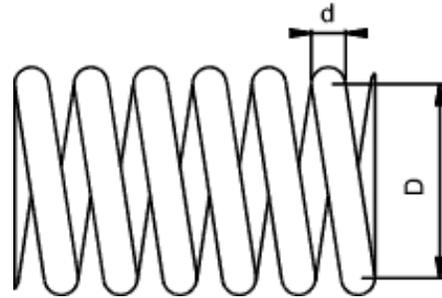
Figure 1. Parameters of a helical spring.
