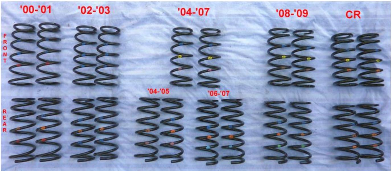
Figure 5. Photograph of the Honda S2000 OE coil spring components used for measurement.
