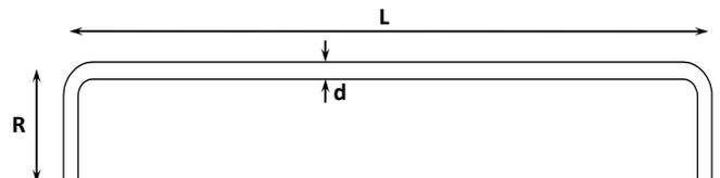
Figure 2. Parameters of an ideal torsion bar
