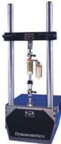
Figure 1 – Shock Dynamometer
